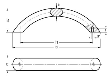
$$\begin{array}{ll} a & = 17 \\ b & = 26 \\ d1 & = M8 \\ h1 & = 57 \\ l1 & = 160 \\ l2 & = 190 \\ t \ min = 12.0 \end{array}$$
